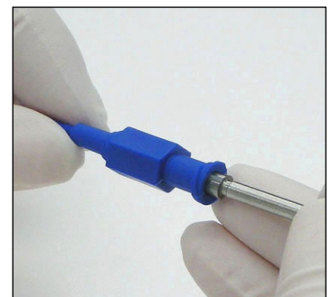
Our Luer testing per ISO 594-1 and ISO 594-2 conforms with required ISO and FDA standards.
